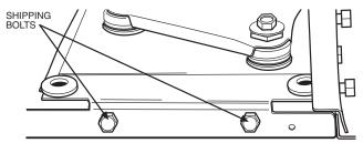
Fig. 15 — Remove 4 Shipping Bolts on Compressor Isolator Plate
